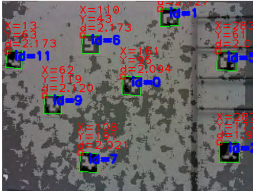
Figure F.10: Measurement vectors printed next to detected ArUco markers within a combined visualization of the RGB and depth image
