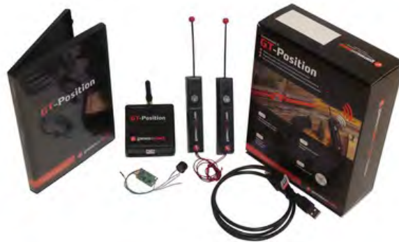
Figure C.1: GamesOnTrack system showing two satellites and one beacon [6]
