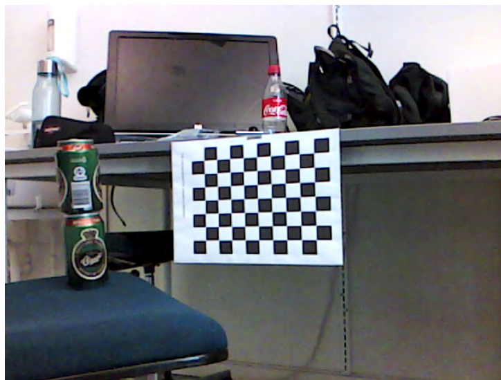
Figure F.4: Example of non-rectified, raw and hence distorted RGB image at 640 \times 480 resolution
