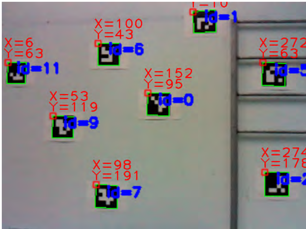
Figure H.5: Implementation of the ArUco markers detection is done in ROS. ArUco markers are printed and placed in the walls. The image shows the detection and identification of some of the markers placed in the laboratory. The implementation streams the marker identifier and its pixel position for visualisation purposes.
